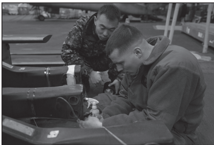
U.S. Marine Corps Cpl. George L. Seely, right, a flight line mechanic with Marine Medium Helicopter Squadron (HMM) 262, 31st Marine Expeditionary Unit, and Navy Aviation Machinist's Mate Wei Wang replace a tip light wire on a rotor blade of a CH-46 Sea Knight helicopter in the hangar bay of the amphibious assault ship USS Essex (LHD 2) in the Pacific Ocean March 29, 2011. Essex was operating off the coast of Japan in support of Operation Tomodachi earthquake and tsunami humanitarian relief efforts. (U.S. Marine Corps photo by Lance Cpl. Brennan O'Lowney)
